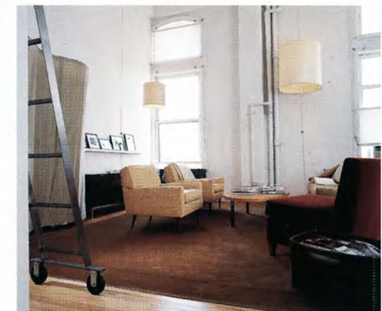
ABOVE "Making room" sometimes means tearing an existing room apart. As part of her campaign to reclaim every inch of usable space, Goolrick stripped off wallboard that disguised utility stacks but took up precious floor area. A partial second floor that sliced through the bedroom/library was also removed.
